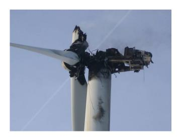
Fig. 2: Burnt down nacelle of a 1.5 MW wind turbine (Image source: Allianz)
